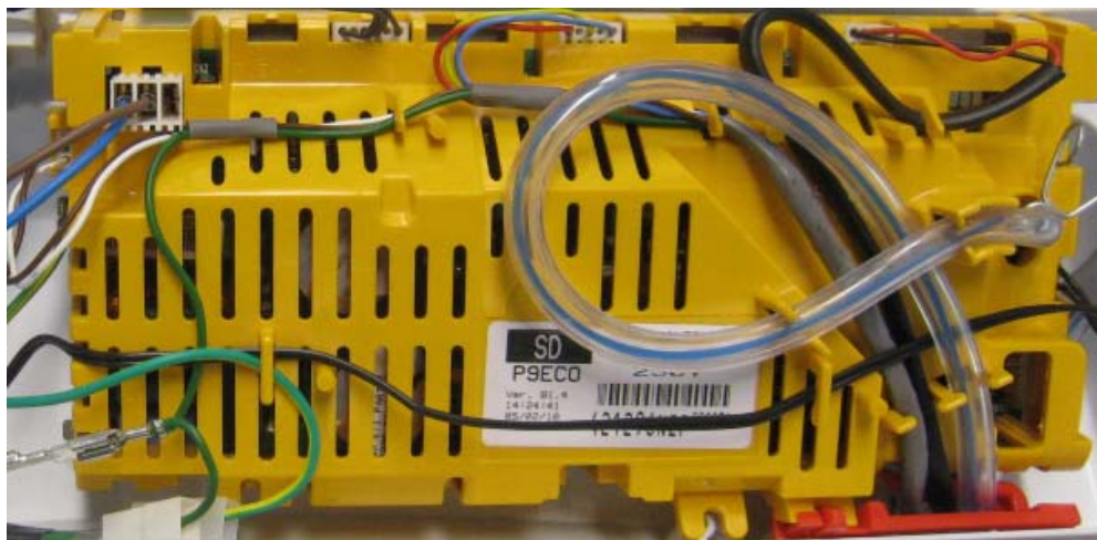
Motor Control Module
