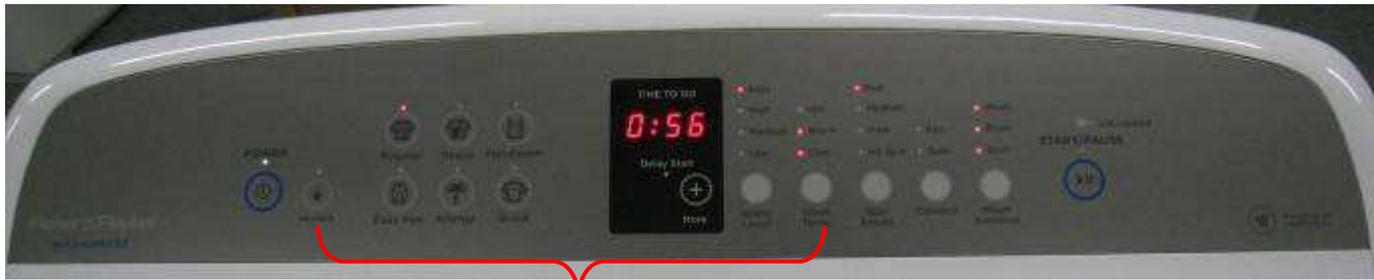
With the console **On** Press & Hold **Key Lock** and **Wash Temp** for 3 Sec. **Diagnostic**
