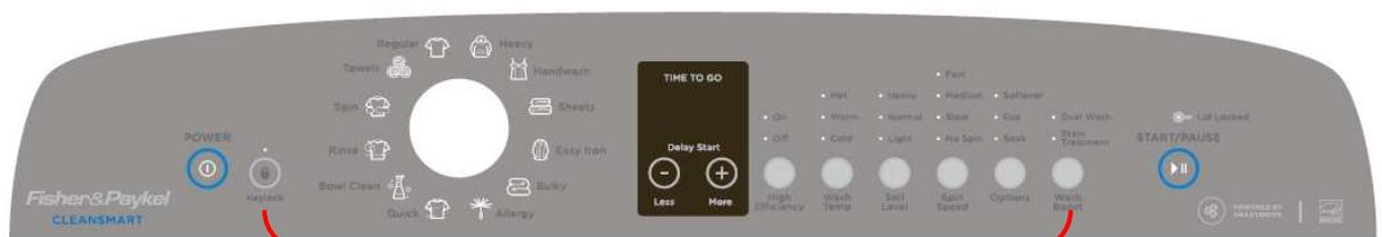
With the console **Off** Press & Hold **Key Lock** and **Wash Boost** for 3 Sec. **Showroom Mode**
