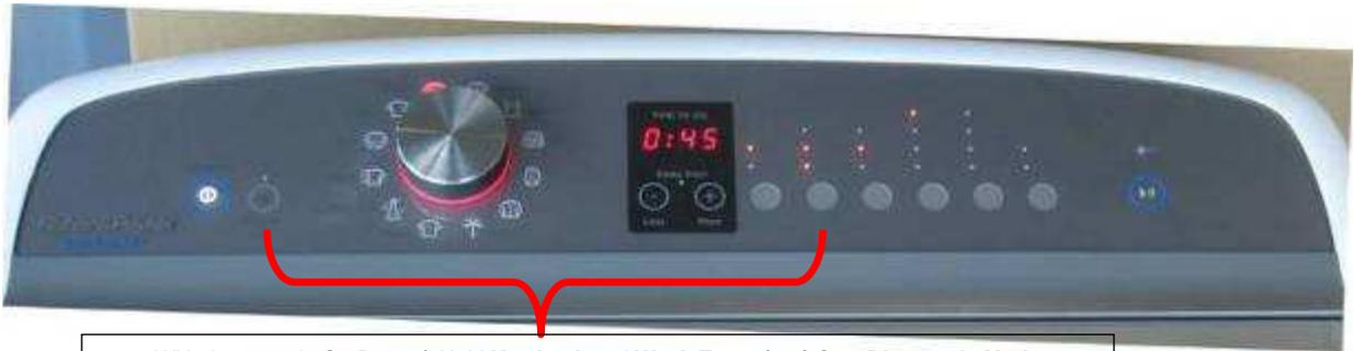
With the console On Press & Hold **Key Lock** and **Wash Temp** for 3 Sec. **Diagnostic Mode**
