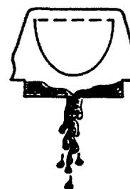
For the Delicate and Permanent Press cycles the fabric softener remains in the dispenser cup throughout the wash and first deep rinse. SmartDrive<sup>®</sup> then spins to release the fabric softener, delivering it down the agitator stem as SmartDrive<sup>®</sup> fills for the final rinse.
