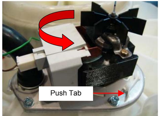
**Note: Approximately 250mls of water remains in the pump sump after pump out and will spill when the pump is removed. Take care not to spill this water over electrical connections by using a towel or small container to catch the water.**
