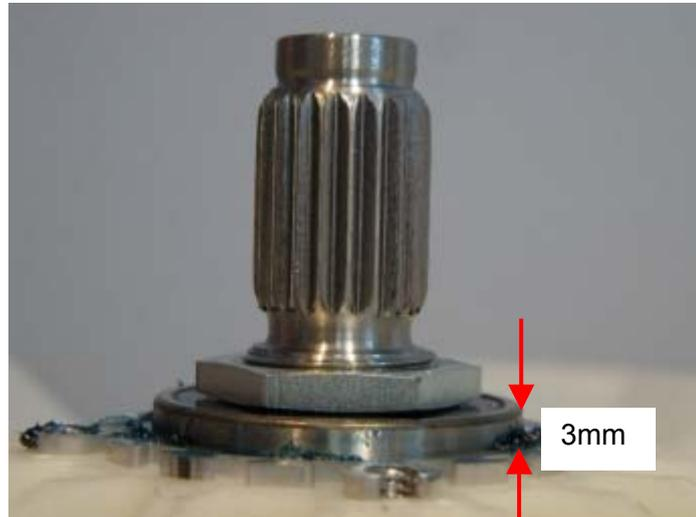
*Note: The outer bearing will be proud of the housing by approximately 3mm.*
