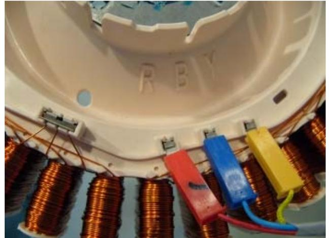
**Note: The Stator should have a slight radial movement of approximately 0.5 – 1mm when correctly tightened, and should have a maximum axial (rocking movement) of 0.5mm.**
