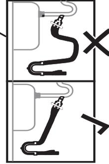
Ensure drain hose is routed straight to joiner. Remove excess drain hose material if necessary. Do not shorten the inlet hose.
