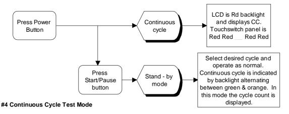
Once a mode has been entered, press Power to exit diagnostics except Display and Show Off modes) which require the plug to be removed from the power socket.
