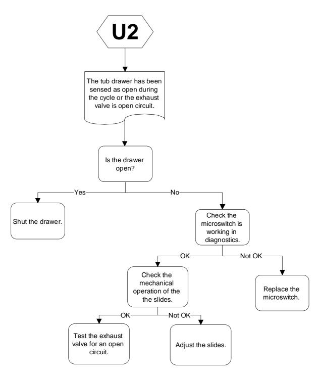
**Note**: Tub home microswitch is located on the rear of the left slide runner and is connected in series with the exhaust valve.
