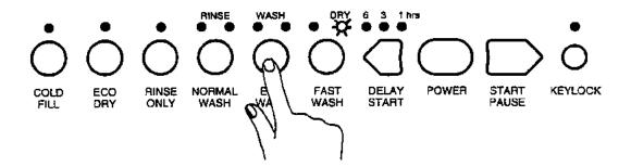
Press the **NORMAL WASH** button. This will activate the drain pump. The Second Fast Wash LED ceases to blink but remains on.
