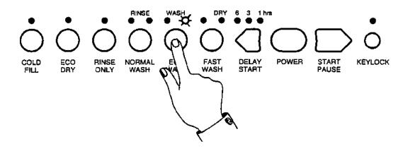
Press the **NORMAL WASH** button. This activates the wash pump. TheSecond Normal Wash LED ceases to blink but remains on. Use an amp meter to check current draw.
