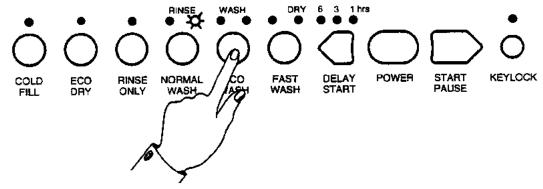
Press the **NORMAL WASH** button. This activates the element. The Second Rinse LED ceases to blink but remains on.
