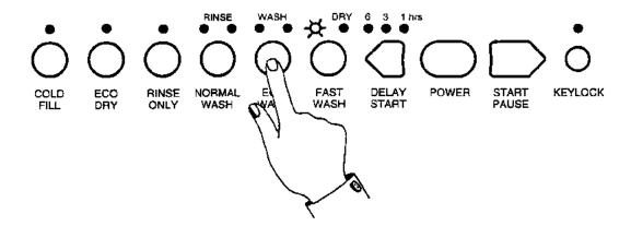
Press the **NORMAL WASH** button. This will activate the detergent dispenser. The First Fast Wash LED ceases to blink but remains on.
