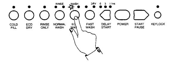
Press **NORMAL WASH** button. This activates hot water valve. First ECO Wash LED ceases to blink but remains on. **Note:** Should tub be full of water, the water valve will not energize due to the pressure switch having already been activated.
