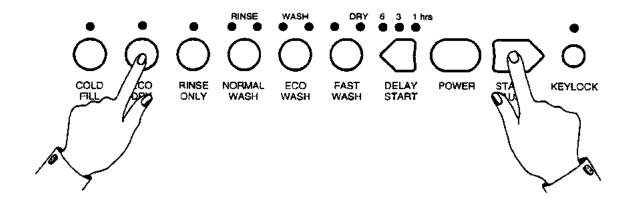
All LED's should be on. Should any fail at this stage it will indicate a faulty LED. A replacement console assembly must be fitted. To exit, press **POWER** button.
