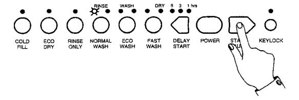
**Note:** To return to the previous tests, press the **START/PAUSE** button once for temperature test, twice for LED display, three times for input test. The water valves will not operate if the machine is full of water.
