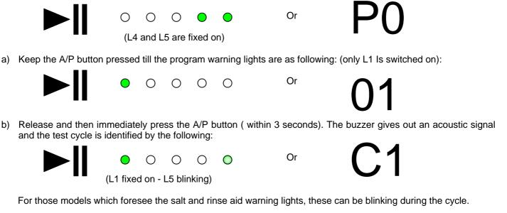
If the test cycle procedure isn't correctly done, it's necessary to repeat the procedure starting from the point (a).
