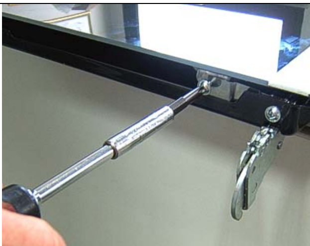
8. Fix the outer glass on the new stirrup.
