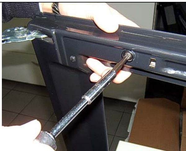
5. Screw the second fixing point of the hinge.
