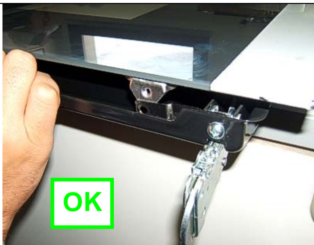
7. CORRECT OUTER DOOR GLASS POSITION (inside the new stirrup )
