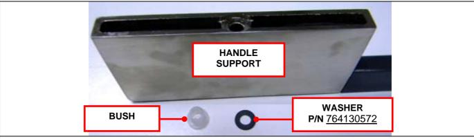
2. Add a washer p/n **764130572** between the handle support and the bush ( for both supports) in order to align the bush base to the handle support edge.
