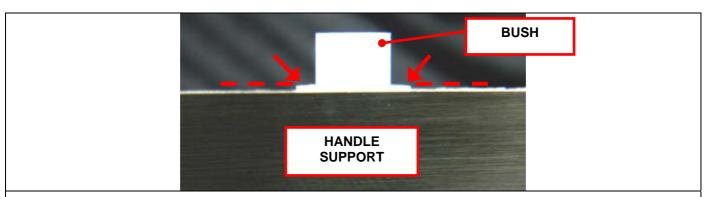
5. Side view of the bush fitted into the handle support.
