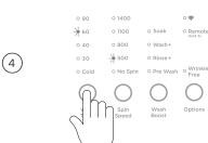
Select your desired wash cycle by turning the Control Dial. The wash cycle icons will illuminate as you turn the dial showing which cycle is selected, along with the default wash cycle settings.
