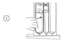
To remove the liquid detergent compartment, firmly grasp and twist the left hand side of the internal compartment and pull upwards.
