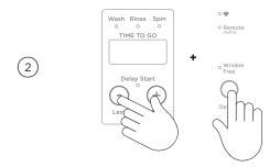
Press **MORE** + , LESS - and **OPTIONS** buttons together for three seconds, dEF will appear on the screen and the washer will beep. Your washer will now be reset to factory default settings.
