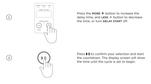
Avoid using DELAY START for damp, non-colourfast items as this may cause dye run to occur.
