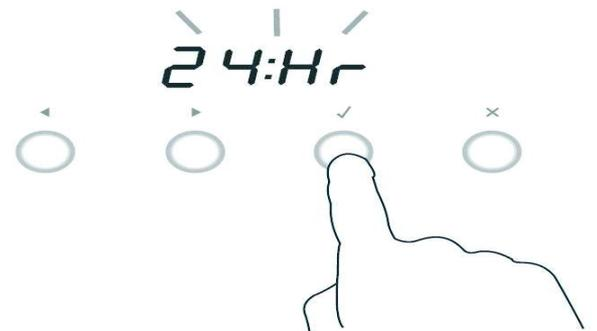
3. Press the right scroll > button on the clock to change between 24 Hr and 12 Hr, then press the tick button to confirm.
