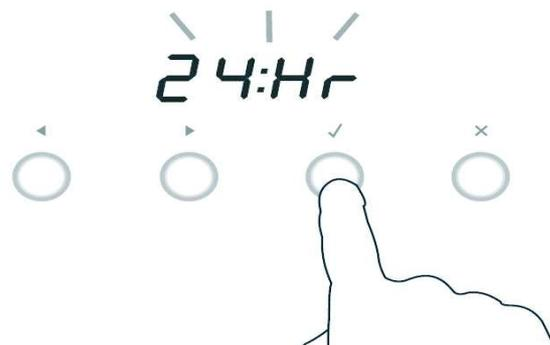
2. Press the right scroll > button on the clock to change between 24 Hr and 12 Hr, then press the tick button to confirm.
