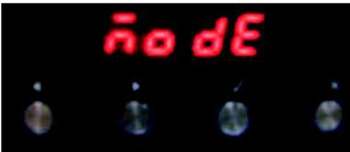
**Note:** If changing a power board or clock module, always check that the correct model ID is set for the product you are working on.
