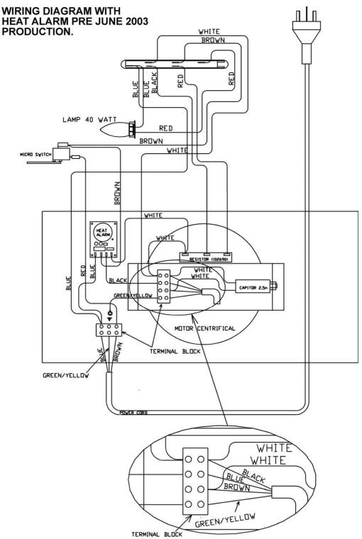
ENLARGED TERMINAL BLOCK TO CLARIFY WIRING COLOURS.
