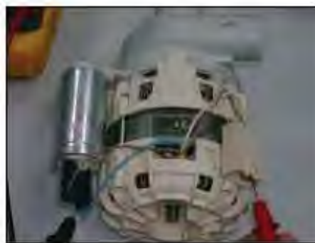
Measurement of the secondary windings of the washing pump (white cable – blue cable)
