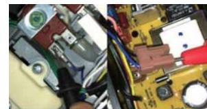
Picture 12.3.1.02 Check the cable connects for the valves.
