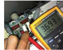
Picture 12.3.1.01 Measure the valve resistance as below picture.
