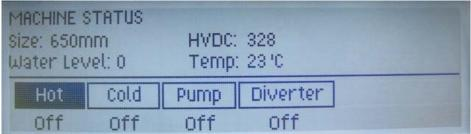
In the top half of the screen it displays the following information. Size is the size of machine, (650mm = Large) HVDC is for on line testing in the factory. WL displays the water level in mm.
