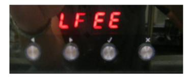
All errors of the Power Board and the Clock Board are displayed using the seven segment digits on the Clock Board.
