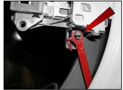
Pull a little of the wiring out of the protection and remove the connector. Disconnect the connector.
