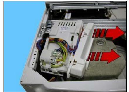
Pull out the connectors positioned beside the board.
