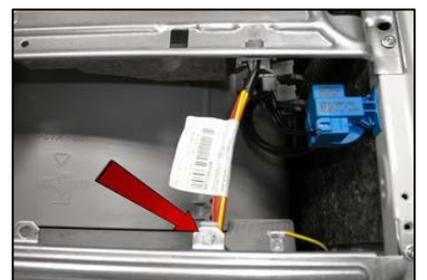
Remove the four screws which secure the crosspiece to the cabinet
