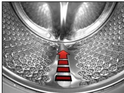
Insert the flathead screwdriver at a right angle to the blade (hole 6), so as to position it at the centre of the two tub tabs.
