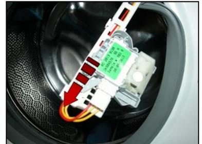
Release the hook, remove the wiring and move it.
