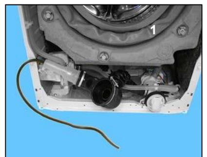
Make a note of the latch and hook with which it is secured to the tub.
