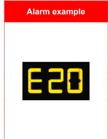
After the problem has been solved, pressing the **Start/Pause** push button the warning message is not shown anymore, buzzer stops the sequence and the cycle restarts.
