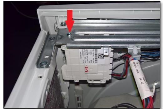
Use a small screw driver to press the tab where indicated by blue arrow then slide the PCB in direction shown to remove.
