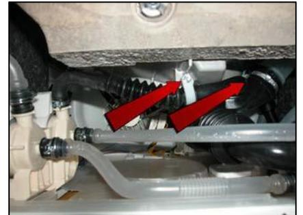
Pull out the main drain pipe (1)
