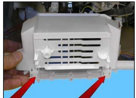
Pull out the wiring from the hooks securing it to the casing of the INVERTER. Remove the connectors.
