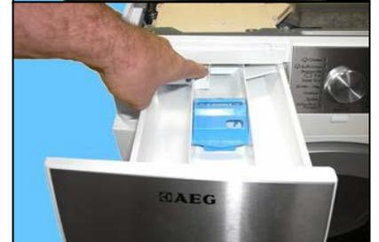
Loosen the screws that attach the control panel to the detergent tray.
