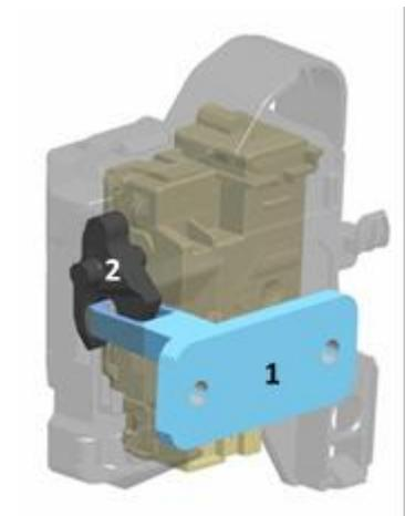
If the appliance is switched off or paused and the appliance handle is pulled, the latch is released from the ratchet (2), effortlessly, whereas if the START/PAUSE button has been pressed, the cursor (8) - being locked - does not allow the ratchet to turn (2) so the fastening latch is locked for the entire wash cycle.
