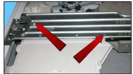
Unfasten the screw in the clamp that fixes the detergent loading pipe to the tray, and remove it from its housing.
