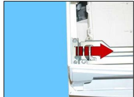
Raise both sides of the control panel so as to pull out the hooks which secure it to the front panel.
