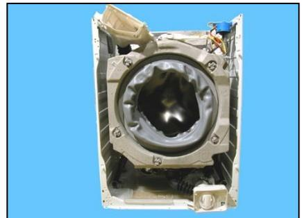
When re-assembling the front panel make sure the small rod of the door safety device is correctly positioned (see "Door safety device" paragraph).
