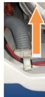
2. Remove the pipe fastener by pressing the hooks (indicated by the arrows) and pull it out at the same time.
