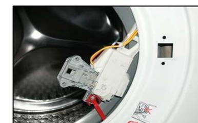
Remove the small rod from the pin (after removal, it stays in the vertical position).
