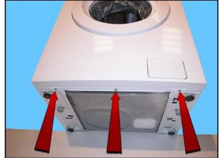
Remove the four screws which secure the front panel to the sides.
