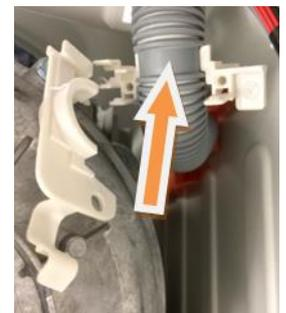
3. When refitting the pipe, make sure that the non-corrugated part is inserted in the seat of the pipe fastener.
