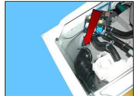
If the appliance is a Jet System, pull out the pipe from the detergent dispenser hook
