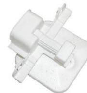
*In the bottom of the washing machine there is a plastic bottom that forms a container. This collects any water leakage (from the tub, from the pipes, etc.), which flows into the area in which the float is positioned (made of polystyrene). In the presence of water this lifts up and triggers the micro-switch, which powers the drain pump.*
