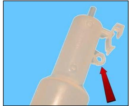
Use a screw Code 405 50 33-52/8 (AF/2P 5x16 TE/SP must have a maximum length of 16 mm and without a tip to avoid perforating the tub), secure the chamber to the tub as shown by the arrow in the photo.
