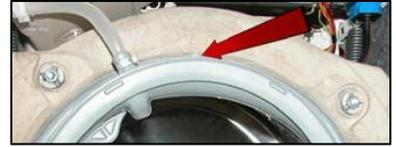
Reassemble the snap ring between the door bellow seal and the tub. Reposition the circulation pipe in its seat.
