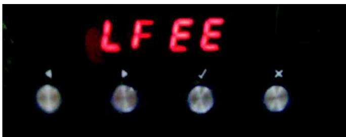
All errors of the Power Board and the Clock Board are displayed using the seven segment digits on the Clock Board.
