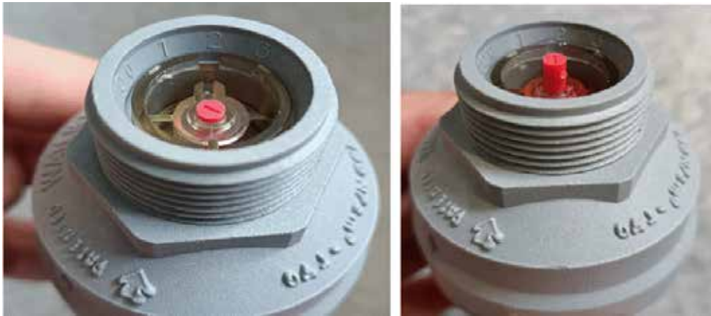
Picture 2 Left: not activated, red cylinder in down position. Right: activated, red cylinder is extended up.
